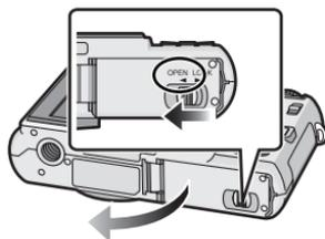
**2** **Battery:** Insert it fully being careful about the direction you insert it. Pull the lever **(A)** in the direction of the arrow to remove the battery.
