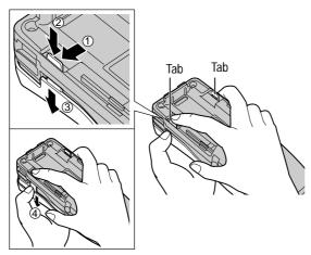
3. Place the new option cover fitting the tabs on the cover into their slots on the handset.
