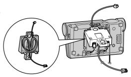
3 Install screws using the wall template below. Connect the Telephone line cord. Mount the unit, then slide down.
