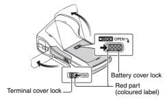
Check that there is no foreign matter on the inner side of the battery cover or terminal cover (where the rubber seal (1) contacts the camera body 2).
