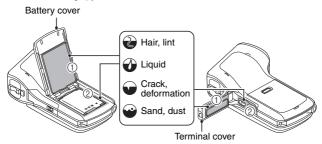
· If the rubber seal inside the battery cover or terminal cover is cracked or deformed, consult the store where the camera was purchased or a nearby service centre.
