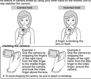
Make sure that the lens and flash unit are not blocked by your fingers or the handstrap. And do not block the built-in microphone on the monitor unit with your hand.
