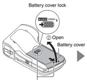
1) Push the battery cover lock to the right to release it.
