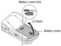
① Push the battery cover lock to the right to release it.
