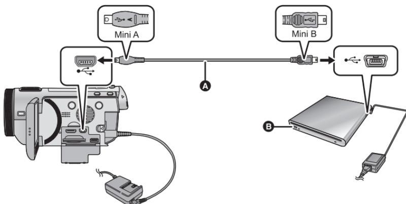
**A** Mini AB USB Connection Cable (supplied with DVD burner)
