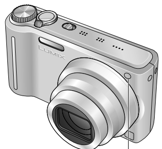
Self-timer indicator (Flashes for set duration)
