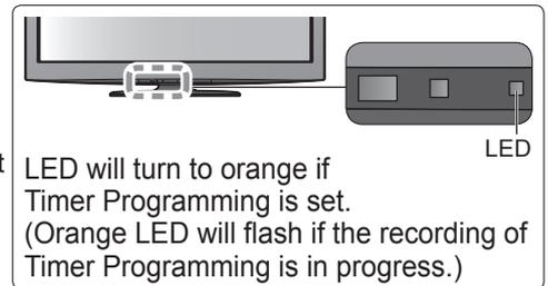
LED will turn to orange if Timer Programming is set. (Orange LED will flash if the recording of Timer Programming is in progress.)
