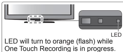
LED will turn to orange (flash) while One Touch Recording is in progress.
