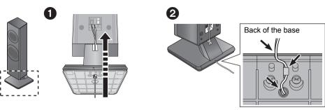
Thread the speaker cable. Use suitable speaker cables for each speaker type. (—STEP4)
