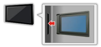
• Remove the CI module from the TV when placing the TV facing upward. This may cause damages to the CI module and CI slot.
