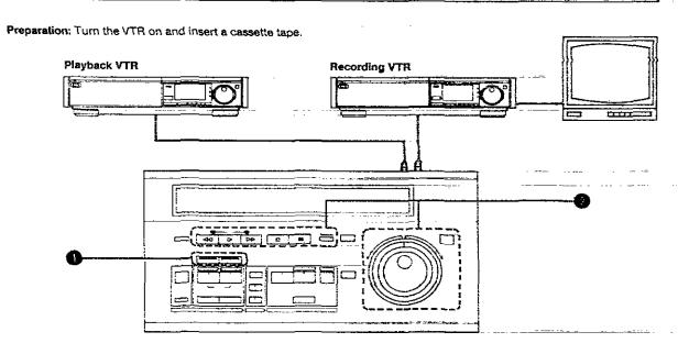
Press the Player Button or the Recorder Button to choose the VTR that you want to operate. To operate both the playback and the recording VTR, press the two buttons simultaneously.
