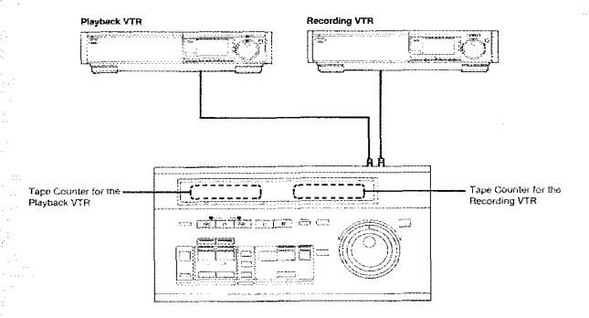
The Counter Indication of the VW-EC310E also works as a lap time counter the indicated elapsed tape time is based on the recording time (hour, minute, second).
