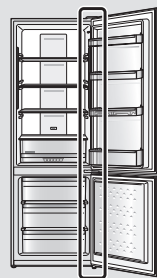
Potential pinch point
