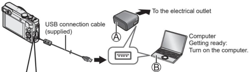
When charging the camera, connect the USB connection cable (supplied) to the [AV OUT/DIGITAL] socket.
