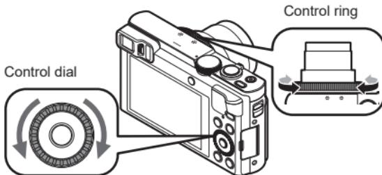
Items that can be set by the control ring/control dial vary depending on recording modes. Following are the pre-assigned settings.
