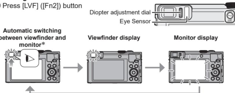
\*For automatic switching between the viewfinder and monitor, the eye sensor automatically switches the display to viewfinder when your eye or an object moves close to the viewfinder.
