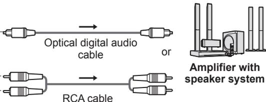
To enjoy the sound from the external equipment in multi-channel sound (e.g. Dolby Digital 5.1ch), connect the equipment to the amplifier. For the connections, read the manuals of the equipment and amplifier.
