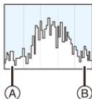
• A histogram is a graph that displays brightness along the horizontal axis (black to white) and the number of pixels at each brightness level on the vertical axis.
