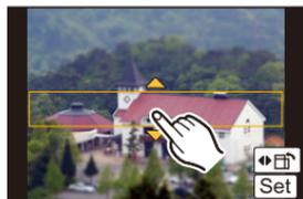
**3 Rotate the rear dial to change the size of in-focus portion.**
