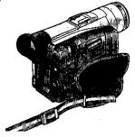
Fold the end of the Shoulder Strap back, pull it first through the loop and then the Shoulder Strap Length Adjuster. Pull it out more than 2 cm 1 from the Shoulder Strap Length Adjuster so that it cannot slip off.
