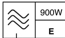
The IEC (705) power output (watts)\*
