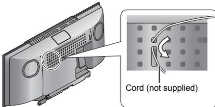
**6** Hook the unit securely onto the wall mount brackets with both hands.
