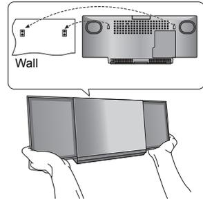
**7** Drive the safety holder fixing screw (not supplied) to secure the safety holder onto the wall.
