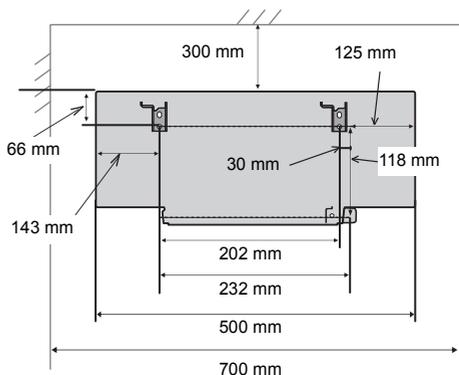
**3** Attach the wall mount bracket to the wall with 2 screws (not supplied). (Both sides)
