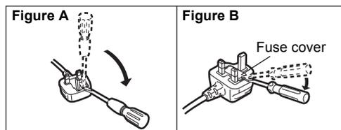
2. Replace the fuse and close or attach the fuse cover.
