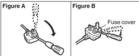
2. Replace the fuse and close or attach the fuse cover.
