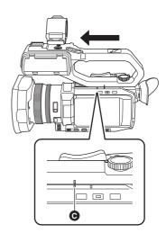
5 While pressing the handle unit mounting screw down, turn it in the direction indicated by arrow ❷ until it stops.
