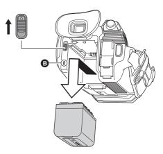
Move the battery release lever in the direction indicated by the arrow and remove the battery when unlocked.
